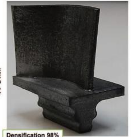
a) Target post sintering geometry b) Spark plasma sintered turbine blade
