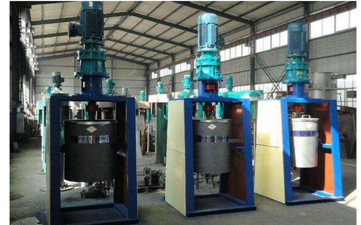
Example of large-scale batch attrition milling
